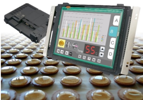
Picture 2+3: With the addition of an adhesive film that overlaps onto the machine panel, the new Open Frame GOT2000 models offer IP67 protection at the front, meeting the needs of hygiene sensitive applications in the food and pharmaceutical sectors.
